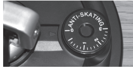
Setting the anti-skating control to zero
