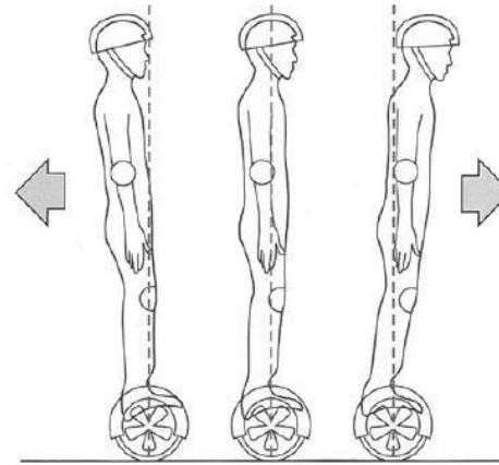
The scooter has a built-in inertia stable system that keeps the balance of forward and backwards directions, but can not assure the stability of left and right directions. Therefore, do not turn around rapidly in high speed, to avoid dangerous situations. Do not shift laterally or turn direction on the slope: it will affect the scooter balance equilibrium angle.
